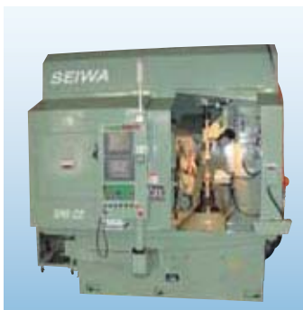
圆柱齿轮CBN磨床 SRG22 清和 SEIWA CBN Cylindrical Gear Grinder SRG22
