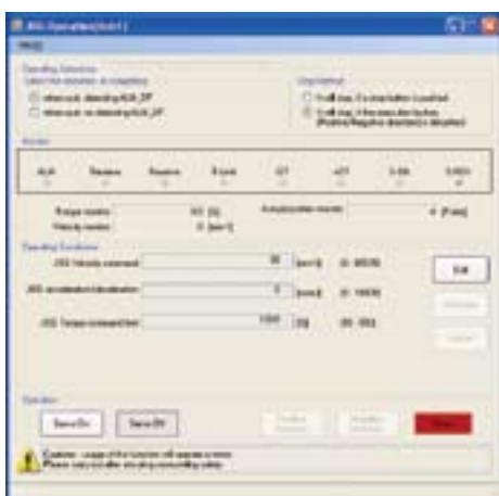
JOG Operation Can simplify servo motor test runs by entering the speed commands from a PC.
