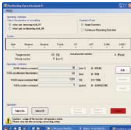
Positioning Control Operation Position can be moved by setting the feed velocity and pulse number of the servo motor.
